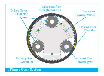
Reducing the flow channel dimensions or closing them totally, applies torque and brakes the system. The images below show how the pressure builds up in the system as the valves are closed. Variable braking torque can be achieved by adjusting the channel width through the positioning of the valves. The TfI design encloses the entire system inside a single annulus gear thus optimising its size and form and delivering maximum performance for minimum volume.
